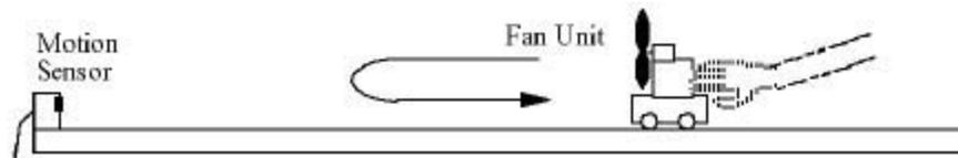
**Figure 1. Typical setup of a MBL-experiment. A low-friction cart is pushed towards a motion sensor. A fan unit attached to the cart provides an approximately constant force in a direction opposite to the initial movement and the cart will thus change its direction of motion. The results are shown in Figure 2. Note that the fan unit provides a visible force.**
