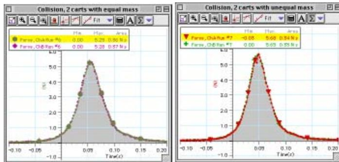
**Figure 3. Results from an MBL-experiment with two colliding carts with equal and unequal masses respectively. Force sensors are mounted on top of each cart. The graphs show the forces measured by the sensors during the collision and the area below curves. Note the time scale. Most students are surprised to discover that the forces are equal when the carts have different masses (see "3rd collision" pre-test in Figure 4).**
