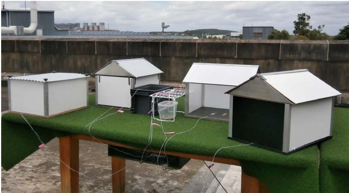
**Figure 3. Structures built for various goals, showing variation in materials and orientation, and use of roof cavity**
