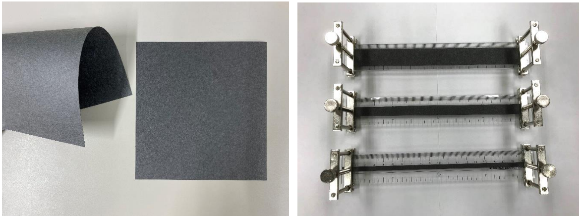
Figure 1. Carbon nanotube paper and the resistors that use it with different widths
