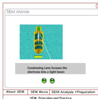
**Figure 3.** Movie created using *Flash MX* showing how the Scanning Electron Microscope works
