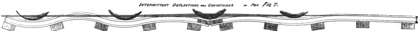
DEFLECTIONS OF SLEEPERS AND SKEW TIES SHOWN THE RAIL DEFLECTIONS ARE ENLARGED 4 TIMES, EVERY FIFTH AND SEVENTH SLEEPER ARE 1
