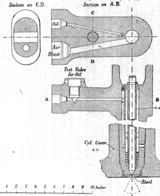
Fig. 6. Oil-spraying Valve.
