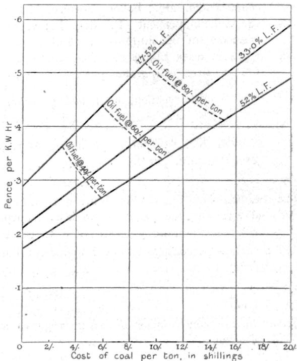
Fig. 10.—Steam Plant. Works Cost—pence per kilowatt-hour Generated.
