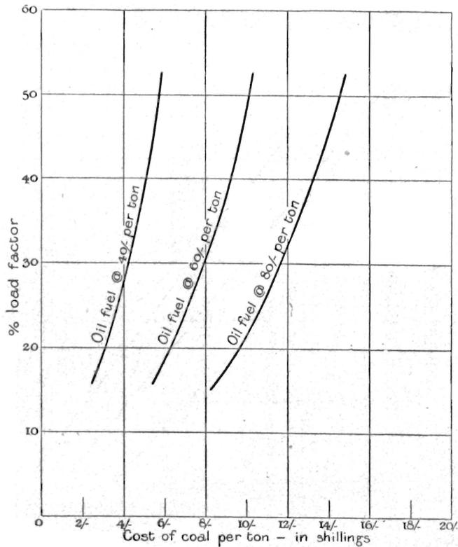
Fig. 12.—Steam versus Oil. Parity Curves.
