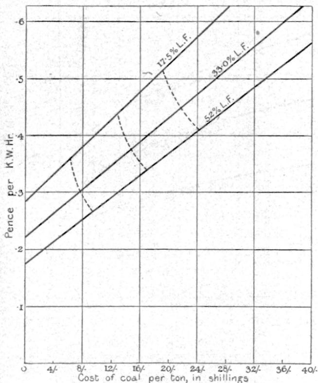
Fig. 11.—Gas Plant. Pence per kilowatt-hour Generated.
