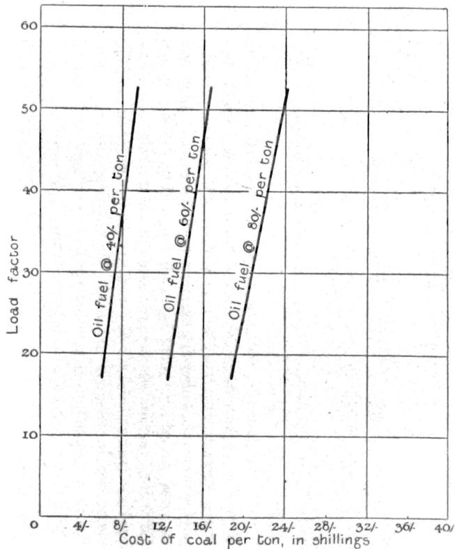
Fig. 13.—Gas versus Oil. Parity Curves.
