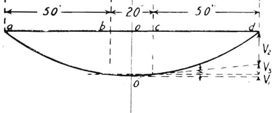
$$\text{Total Deflection} = \Delta = V_1 + V_2 + V_3$$
