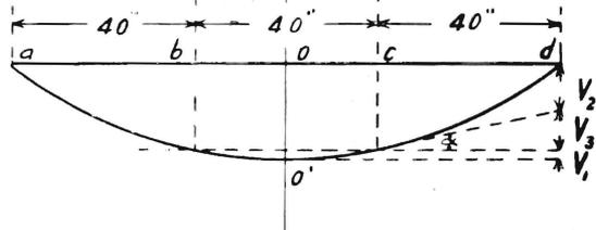
$$\text{Total Deflection} = \Delta = V_1 + V_2 + V_3$$
