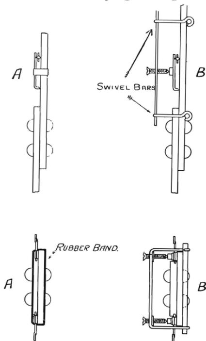
FIG. 18.—Methods of Pressing the Extensometer Against the Test Piece.
