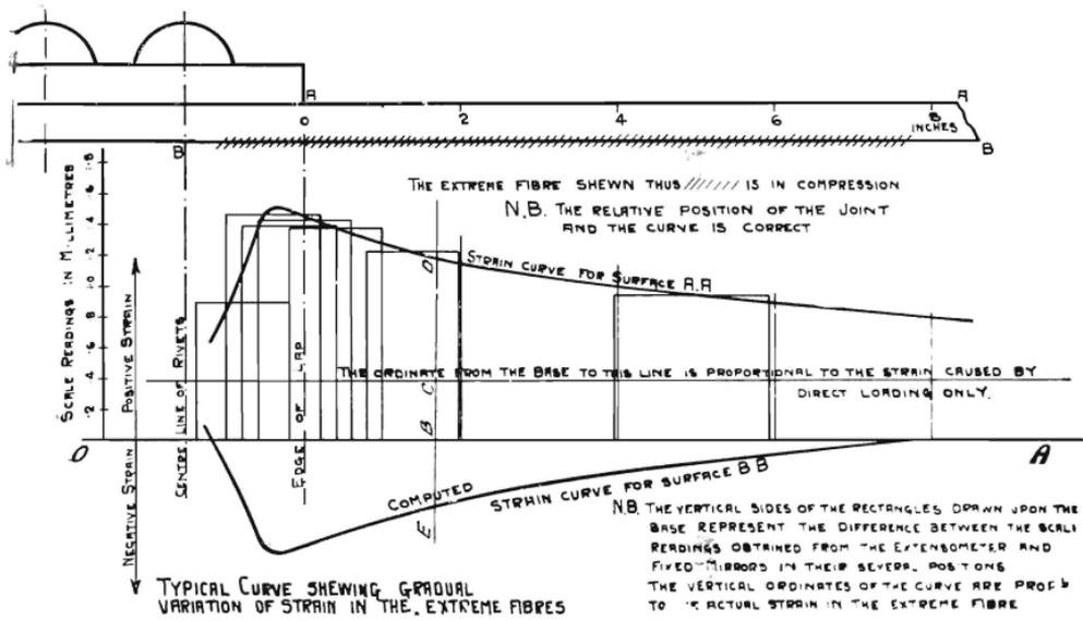
FIG. 21.—Strain Curves for Lap Joints.
