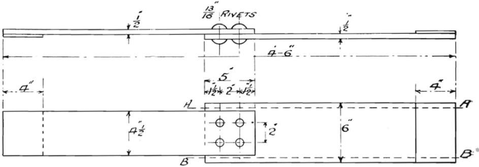
FIG. 16 A. LAP JOINT WITH STRAIGHT PLATES.
