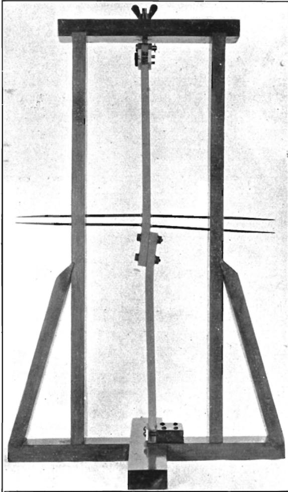
FIG. 21A.—Lap Joint made of Rubber Strips bolted together. Pointers attached to demonstrate the tension and compression. but it is of opposite sign. A rubber model of a lap joint (see Fig. 21A) affords an interesting illustration of this action.
