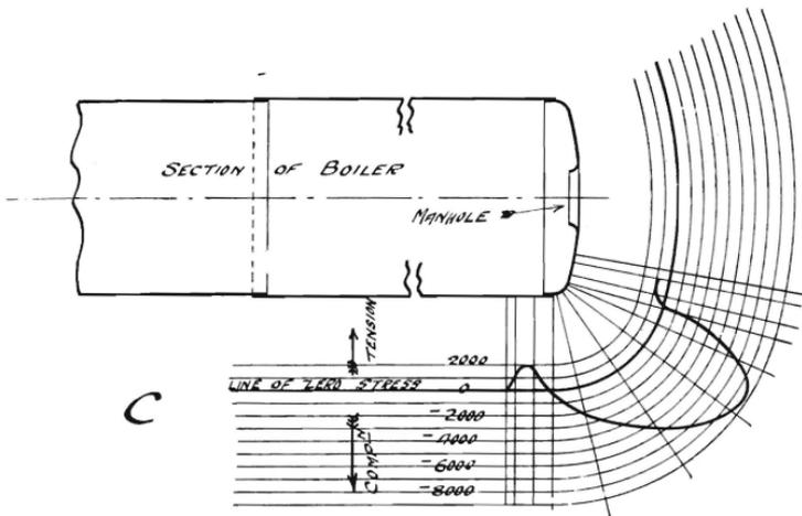
ADDITIONAL STRESSES CAUSED IN THE OUTER EXTREME FIBRES IN THE NEIGHBOURHOOD OF THE DRUM HEAD JOINT OF A B & W BOILER, DEDUCED FROM OBSERVATIONS TAKEN ALONG THE TEST LINE QP WHEN THE COLD WATER PRESS IN BOILER WAS 100 LBS/SQ IN. THE FIGURE GIVES THE EXTREME FIBRE STRESSES AT THE POSITION OF THE EXTREME FIBRES IN WHICH THOSE STRESSES OCCUR.
