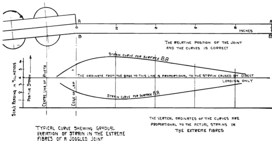
FIG. 22.—Strain Curves for Joggled Joints
