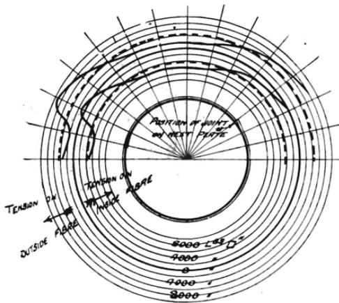
SECTION OF A B & W BOILER BARREL WITH CORRESPONDING EXTREME FIBRE STRESS SECTION ALONG THE TEST LINE A,B. COLD WATER PRESS IN BOILER = 100 LBS/SQ IN. N.B. THE DOTTED LINES REPRESENT WHAT THE EXTREME FIBRE STRESS WOULD HAVE BEEN FOR A JOINTLESS CYLINDER OF THE SAME DIMENSIONS.
