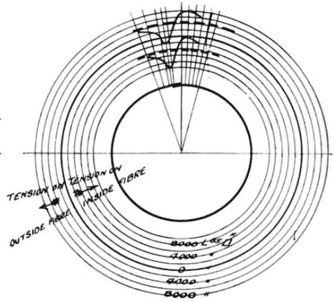
SECTION OF VERTICAL BOILER (HUSKINS) WITH CORRESPONDING FIBRE STRESS SECTION ALONG THE TEST LINE, COLD WATER PRESS = 50 LBS/SQ IN. N.B. THE DOTTED LINES REPRESENT WHAT THE EXTREME FIBRE STRESS WOULD HAVE BEEN FOR A JOINTLESS CYLINDER OF SAME DIMENSIONS.
