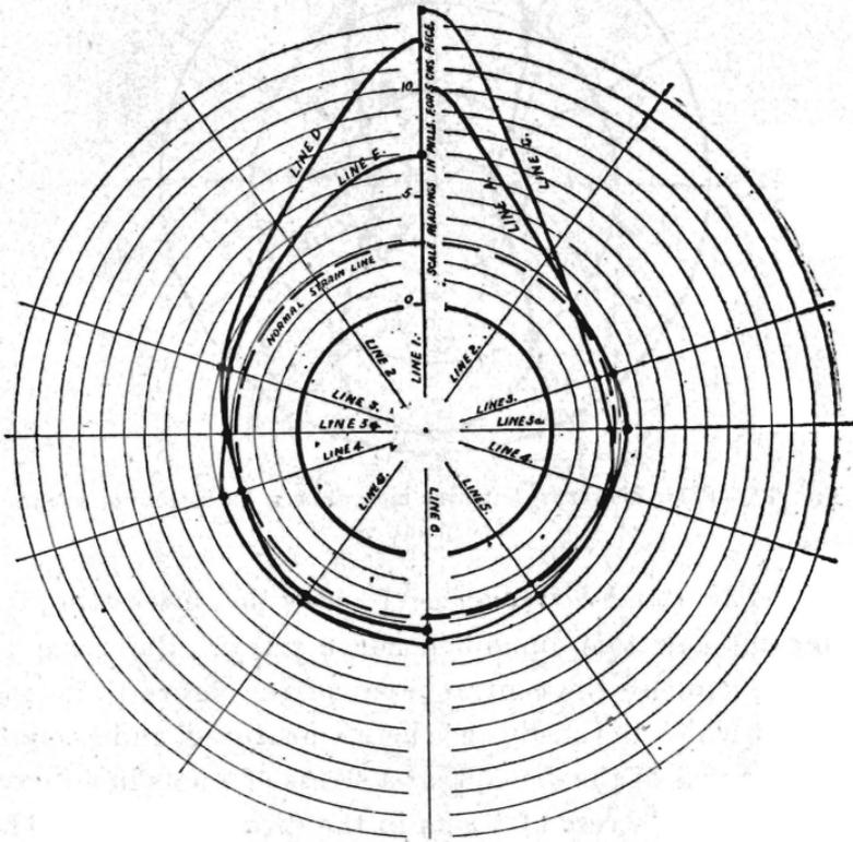
FIG. 12.—Curves of circumferential strain showing the strains measured on lines A, C, D and E.
