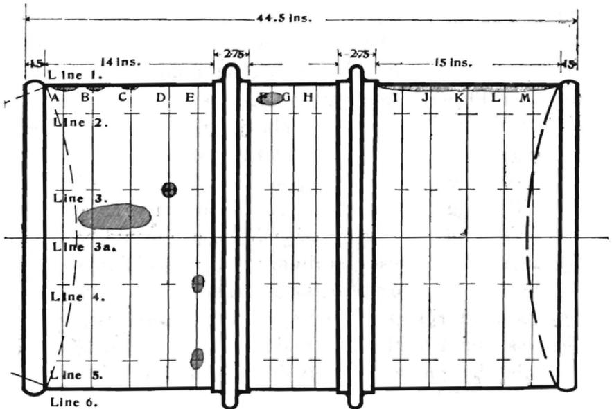
FIG. 7.—Drum F, showing longitudinal test lines 1 to 6, and circumferential test lines A to M. The shaded areas represent the positions of slight dents.
