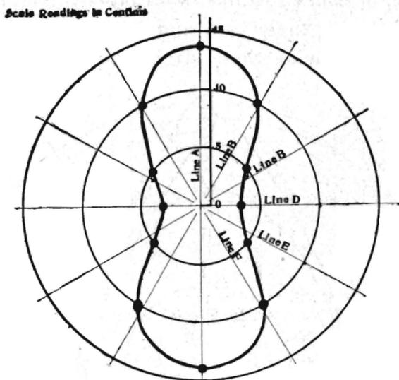
FIG. 13.—Polar diagram of strains measured in all directions round the point G.
