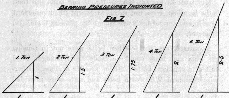
The resultant of all forces was to fall within the centre third of the foundation, and the average pressure was not to exceed half the maximum bearing pressure allowed.
