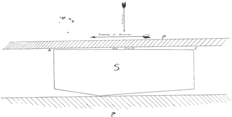
DIAGRAM SHOWING PRINCIPLE OF MICHELL BEARING
