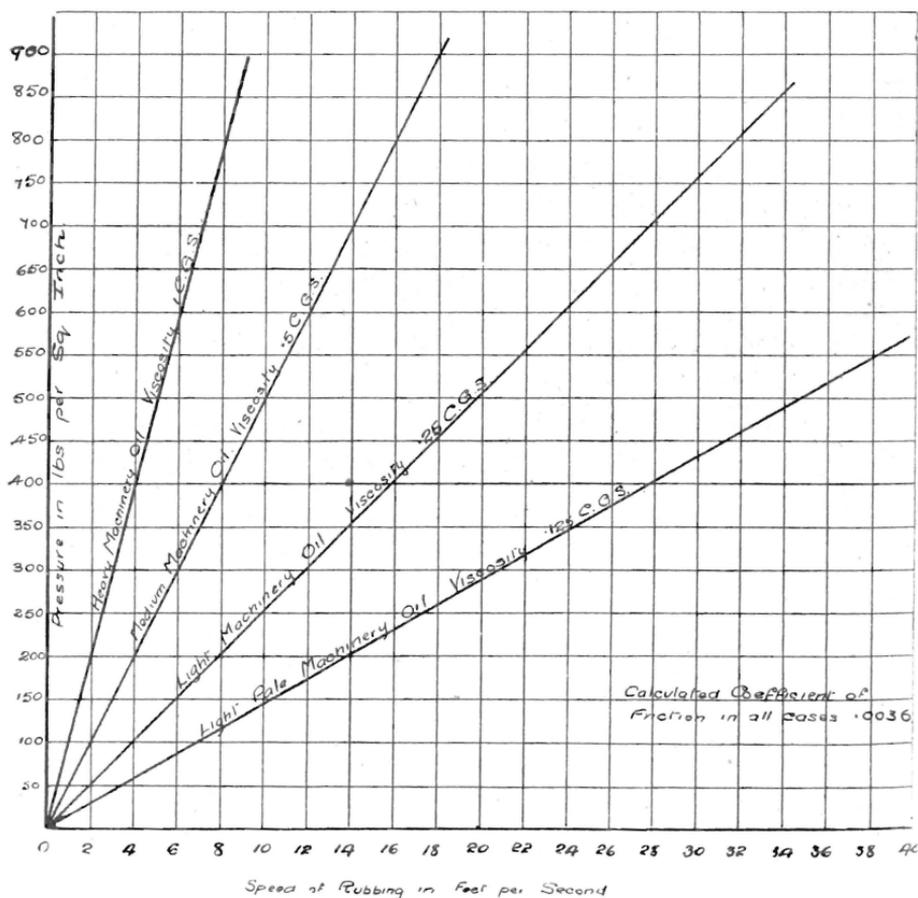
MICHELL BEARING DIAGRAM OF SPEEDS & PRESSURES
