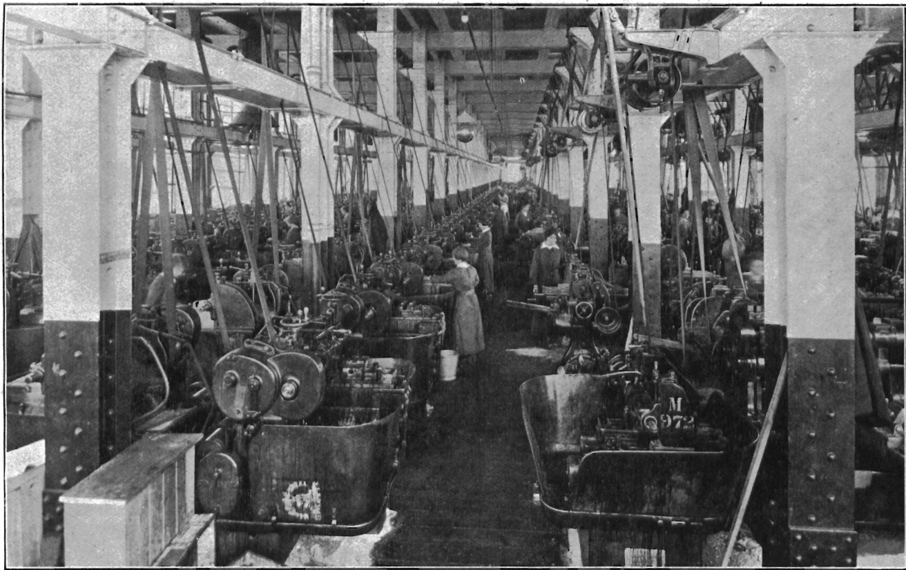
No. 77.—Machine Gun Manufacture. Girls operating cross milling machine on machine gun parts.
