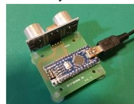
Fig.2 Mobile ultrasonic sensor unit
