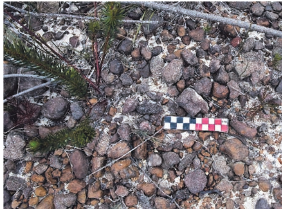
Figure 47. Alleged 'lateritic ironstone.' A surface lag gravel of iron rich sandstone, some with yellow-brown goethite coating. Lambert Peninsula. Scale is 10 cm long.
