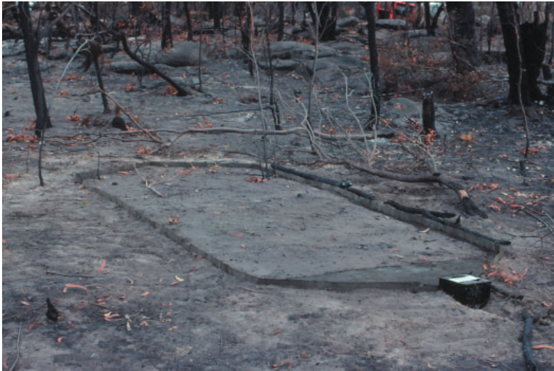
Fig 3. Plot 1, a 9 m 2 closed plot installed on a crest to measure soil loss in t ha -1
