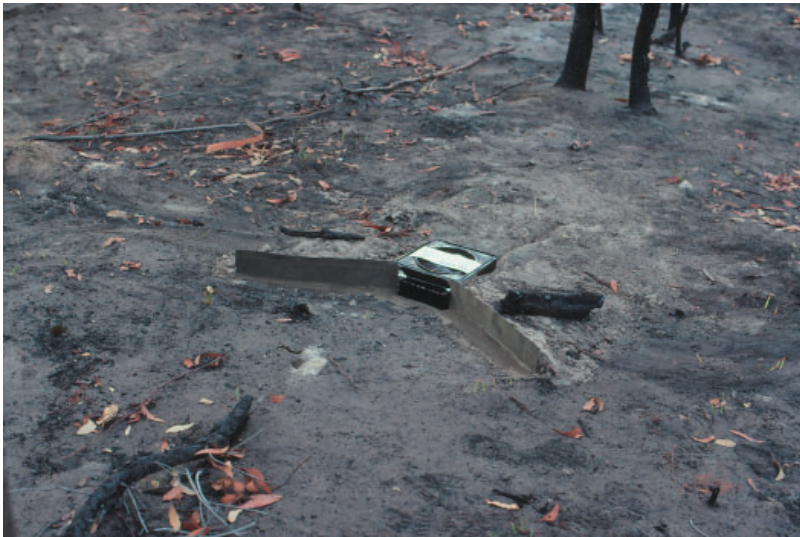
Fig 4. An open sediment trap 1.0 m wide to measure sediment flux
