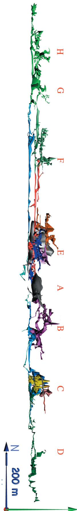
**Figure 2, Long Section, looking east, of the Jenolan Show Caves courtesy of Alan Warild, Jenolan Survey Project. Note regularly spaced high points B-H mostly cupola swarms, separated by zones of generally horizontal development A = Grand Archway, B = Cathedral, Lucas Cave, C = Baal-Orient System.**
