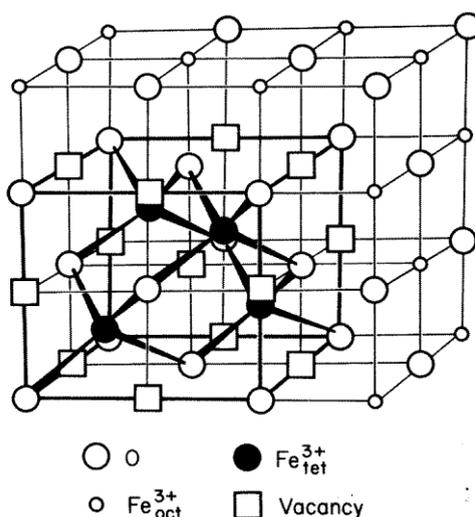
FIGURE 3. Fe<sub>1-x</sub>. Koch-Cohen cluster comprising four tetrahedral iron atoms surrounded by thirteen vacant sites in rock salt structure.
