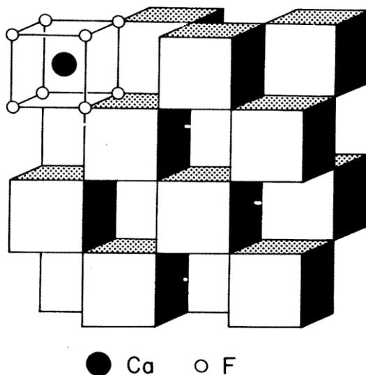
FIGURE 6. Fluorite structure represented as edge-sharing  $\text{MO}_8$  cubes.
