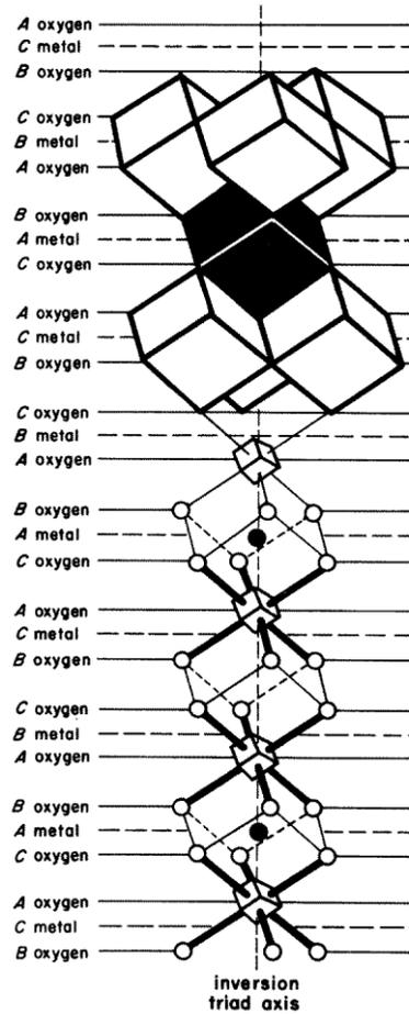
FIGURE 11.  $M_7O_{36}$  defect cluster and the octahedrally coordinated anion vacancies  $\square O_6$  delineated along the same  $[111]_F$  axis.
