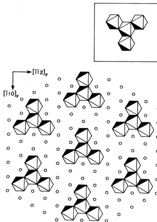
FIGURE 18. Type C- $\text{M}_2\text{O}_3$ . Arrangement of vacant anion sites on a  $(111)_F$  plane showing their coordination octahedra. The  $\zeta$  chirality of the  $\text{Ⓢ}$ -shaped clusters in this plane is contrasted with the  $\Delta$  configuration of adjoining  $(111)_F$  planes shown in the inset.
