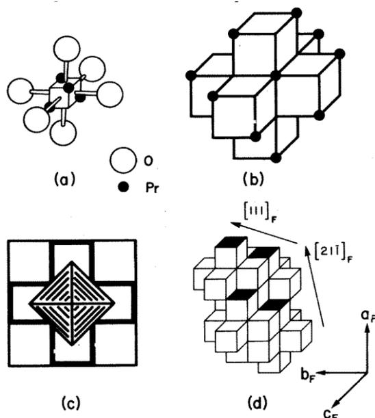
FIGURE 8. (a) Stereochemical environment of vacant anion site; (b) topology of coordination defect with composition  $M_{3.5}\square O_6$ ; (c) octahedrally coordinated anion vacancy  $\square O_6$  in projection on fluorite matrix; (d) cluster of four c.d.s occurring in  $[-Pr_7O_{12}]$  showing important directions.
