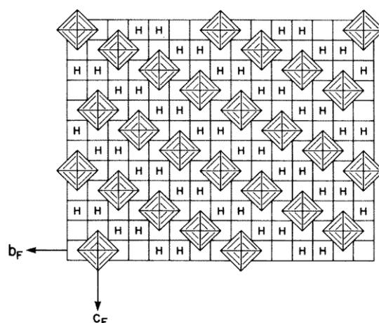
FIGURE 9. Idealized square-matrix representation of a  $(100)_F$  layer of the fluorite lattice showing the location of vacant oxygen sites in  $\bar{1}\text{-Pr}_7\text{O}_{12}$  along  $[0\bar{2}1]_F$  and  $[0\bar{1}3]_F$  directions. Mating holes for accommodating contiguous layers are designated by H.
