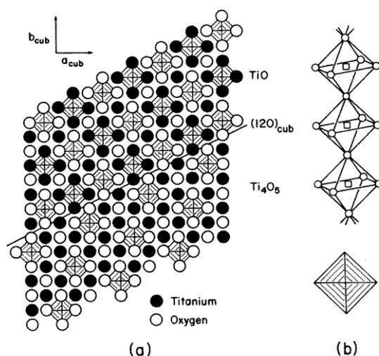
FIGURE 2. (a) The idealized structures of ordered  $\text{TiO}$  and  $\text{Ti}_4\text{O}_5$  coherently intergrown across a  $(120)_{\text{cub}}$  plane of rock salt structure; (b) Vacant cation and anion sites are octahedrally coordinated by oxygen and metal atoms respectively, and occur as extended strings of composition  $\square_{\text{M}}\text{O}_5$  and  $\square_{\text{O}}\text{M}_5$  to yield  $\text{Ti}_{5/6}\text{O}_{5/6}$ .
