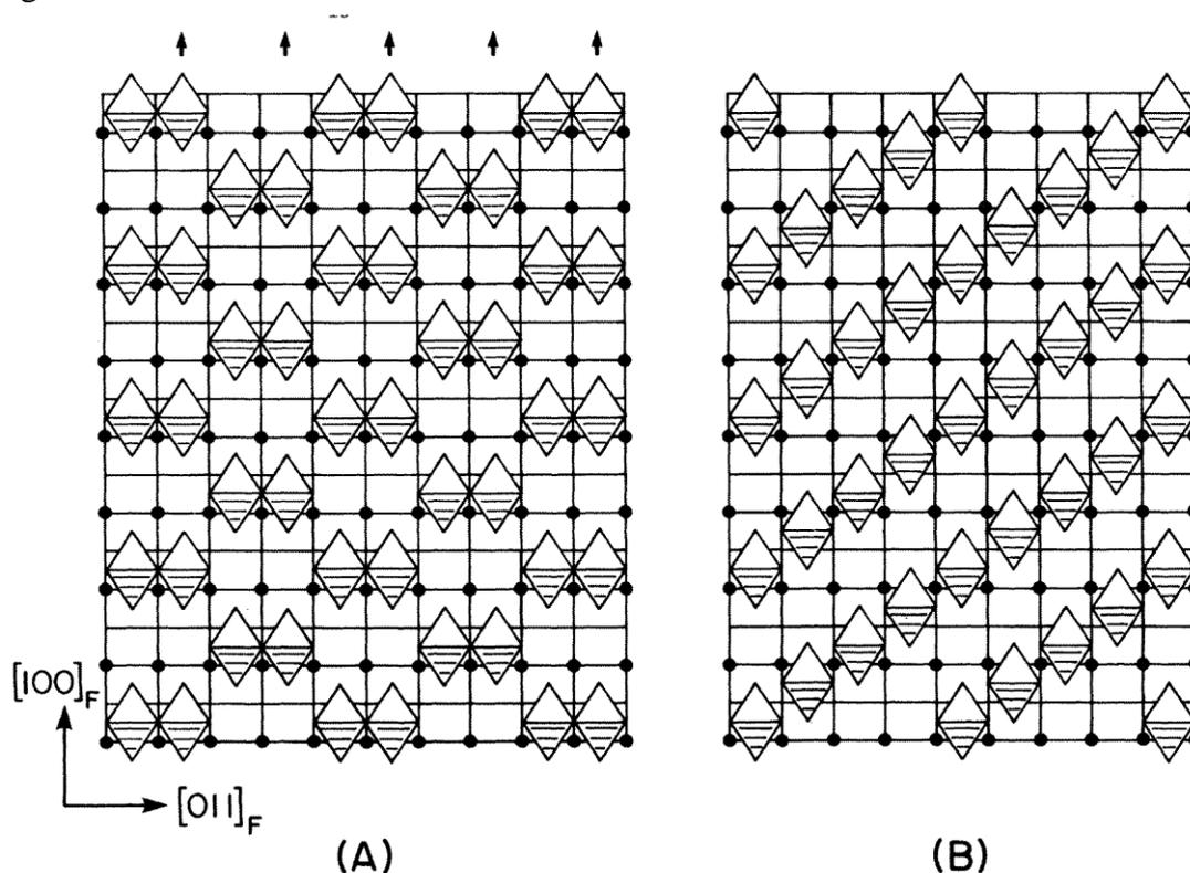
FIGURE 20. Type C- $M_2O_3$ . Two  $(01\bar{1})_F$  planes, denoted A and B, which alternate in the structure. Plane A is converted to plane B by  $a/2$  slip of alternate  $[100]_F$  rows of c.d.s in the direction of the arrows.
