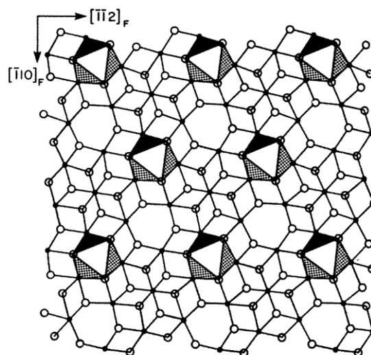
FIGURE 10. Section of  $\bar{1}\text{-Pr}_7\text{O}_{12}$  structure perpendicular to  $[111]_F$  axis. Arrangements of vacant anion sites in a  $(111)_F$  layer is shown by their coordination octahedra.
