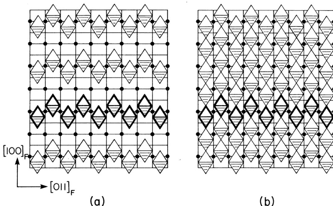
FIGURE 16. Structure of (a) pyrochlore and (b)  $\text{Sr}_2\text{UO}_5$  (or  $\textcircled{R}\text{-Bi}_2\text{O}_3$ ) on an  $(0\bar{1}\bar{1})_F$  plane. The rows of c.d.s along  $[011]_F$  form "extended defects" (outlined), the anion vacancies being related by either  $[111]_F$  or  $[1\bar{1}\bar{1}]_F$  metal-centred vectors.
