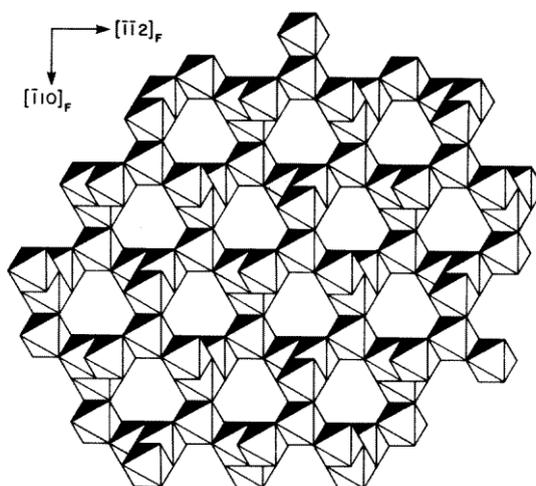
FIGURE 19. Type C- $M_2O_3$ . One of the two interpenetrating networks of c.d.s ( $\nabla$  chirality) showing the edge-sharing involved between planes 1, 3 and 5.
