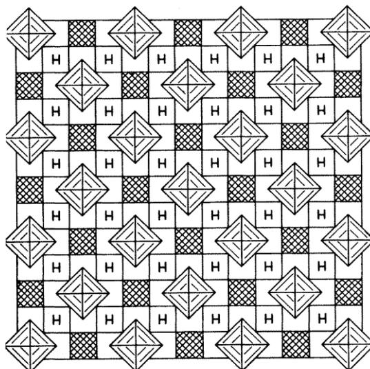
FIGURE 13. Pyrochlore structure  $\text{MgO}_{14}$ . Idealized matrix representation of a  $(100)_F$  layer showing location of vacant oxygen sites as c.d.s. Additional  $\text{M}_{0.5}\text{O}$  octants are cross-hatched.
