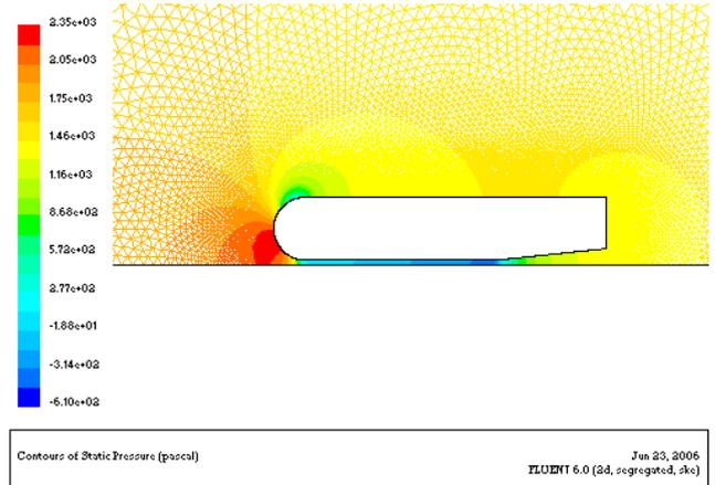
Figure 6: Pressure Contours for 6-Degree Ramp Angle
