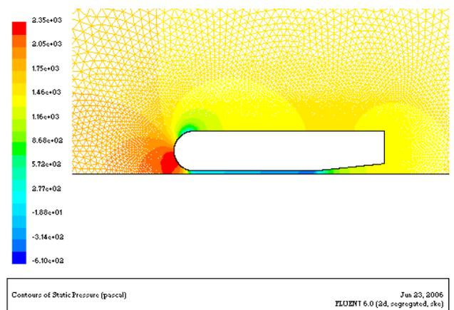
Figure 10: Six Degrees Ramp Angle Pressure Contour Display
