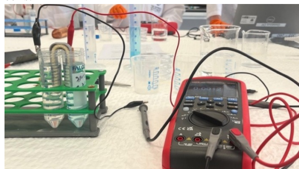
Figure 2: Zinc-Copper Galvanic Cell Experimental Setup
