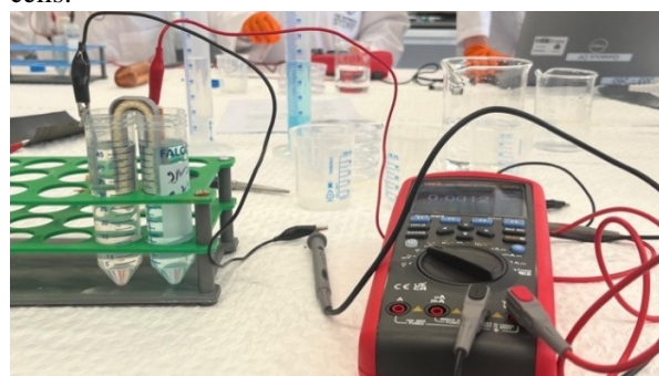
Figure 2: Zinc-Copper Galvanic Cell Experimental Setup
