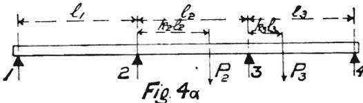
NOTE.—In all cases of continuous girders “ $k$ ” is the distance per unit of length, from the nearest abutment on the left.
