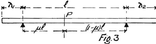
As an extension of Case 2 we could combine the curves of Cases 1 and 2 to treat a beam supported at two points with overhanging ends. (Fig. 3.)
