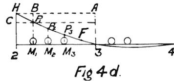
The girders are assumed continuous over three supports on the same level; and the equations as deduced below are got from the equation of three moments, proofs of which are given in many text-books. †
