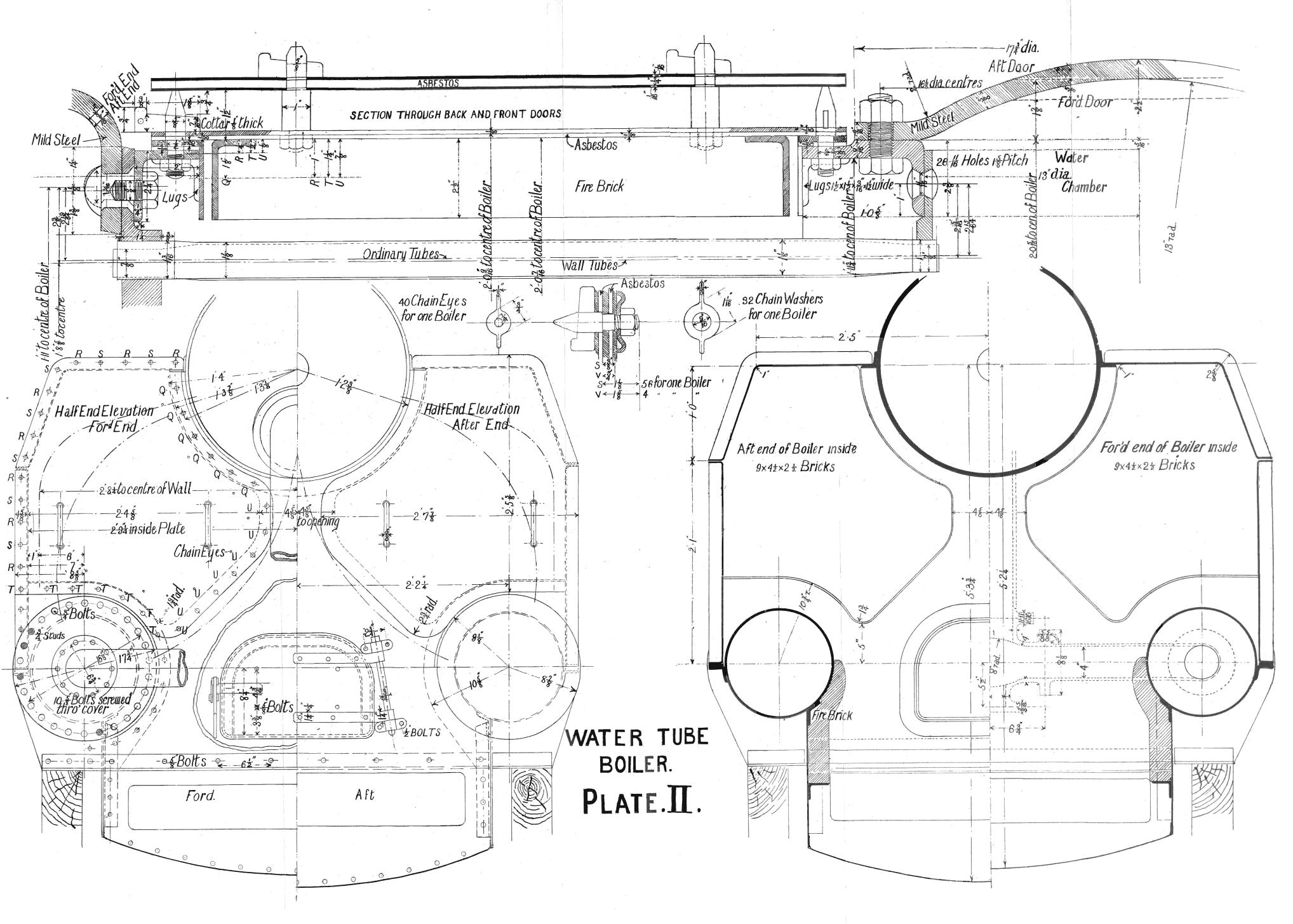
Side Casings.—No brickwork is provided for the side casings, it being assumed that the wall tubes will absorb the greater part of the heat left in the gases, after passing through the nest of tubes. Insulation is however obtained by means of asbestos millboard and air spaces.
