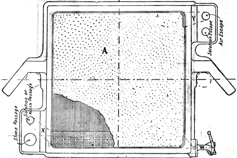
FIG. A.—Solution Plate for Filter-Press.
