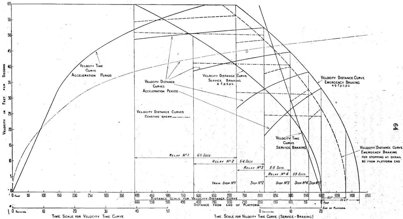
**DIAGRAM** SHEWING ARRANGEMENT OF RELAYS AND TRAIN STOPS NECESSARY TO STOP WITHIN 124.4 FT BEYOND PLATFORM OR TO DERAIL AT 80 FT BEYOND STATION AT 13.6 M.P.H. MAX. SPEED.
