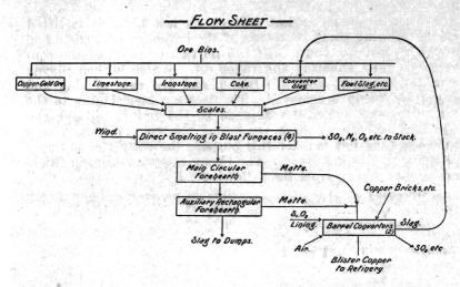
The recovery of copper is about 88-89 per cent. The loss in slags, 10 per cent.; and unaccounted for, probably up the stack, 1-2 per cent. The recovery of gold is about 102 per cent. These figures are based on the actual gold and copper got compared with the amounts said to be present in the ores and fluxes by assay.
