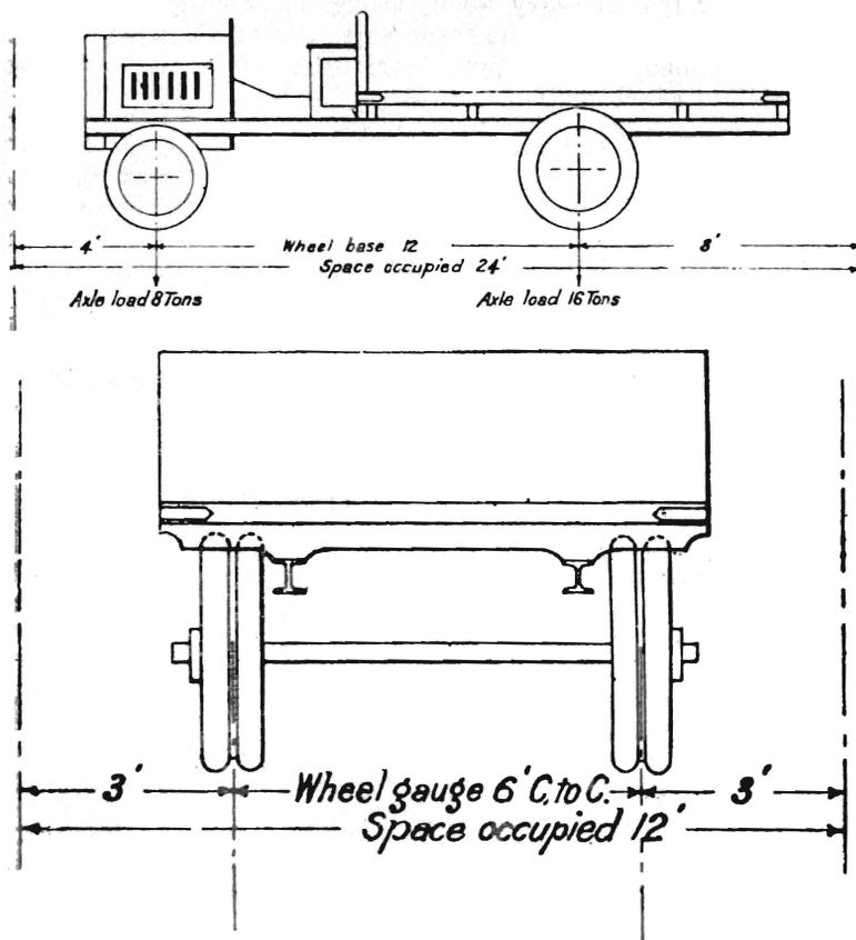
For closely packed heavy vehicular traffic a distributed load of 100lbs. per square foot may obtain over the whole bridge. It is not considered possible that it can be exceeded. The average heavy traffic will be very much less. The high figure was adopted so that no restriction or regulation of the roadway traffic will ever be needed.
