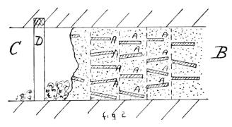
A, A, A, A, etc.—Section of boring holes in tunnel.
