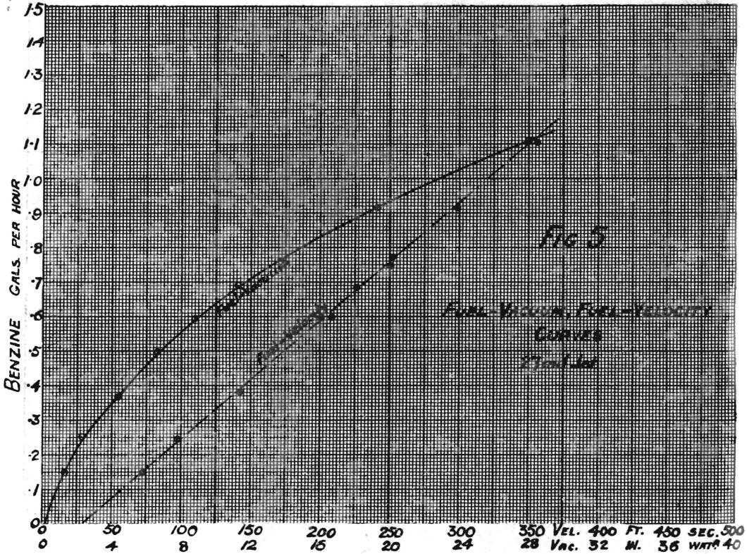
reached, or a corresponding suction-head of  $.2$  in. This is due, as stated before, to the surface tension of the liquid requiring a certain force to break it down, before the liquid can leave the orifice.
