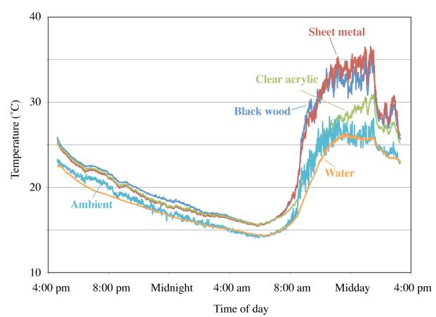
Figure 2. Sample data for the house experiments, showing distinct variations in internal temperatures over 24 hours, for simple model houses constructed from different materials, and for a comparably-sized body of water
