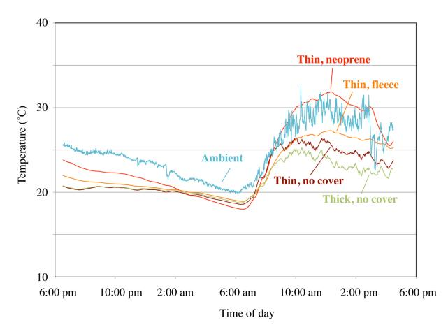
Figure 5. Sample data for the animal experiments, showing distinct variations in internal temperatures over 24 hours, for model animals (cylinders) of different dimensions and covered in different materials – black-surfaced neoprene and sheepskin with fleece attached
