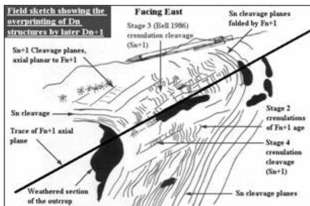
Figure 3. Example field sketch, from the pre-field course section showing the overprinting relationships of the structures
