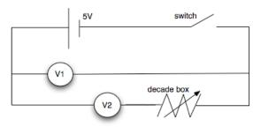
When the resistance of the decade box equals the internal resistance of the voltmeter V2:
