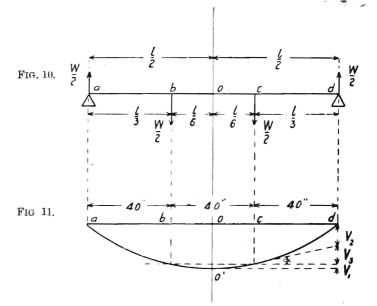
Total Deflection =  $\Delta = V_1 + V_2 + V_3$
