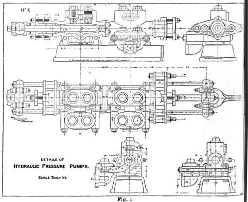
The No. 2 set of pumps is driven by a Phoenix Co.'s Open Type Motor, Compound Wound, fitted with interpoles, and arranged for variable speed work from 300 to 900 R.P.M., the compound winding after starting being cut out when the motor reaches minimum speed. The motor is capable of developing 110 B.H.P. on a 480 volt D.C. circuit, one-
