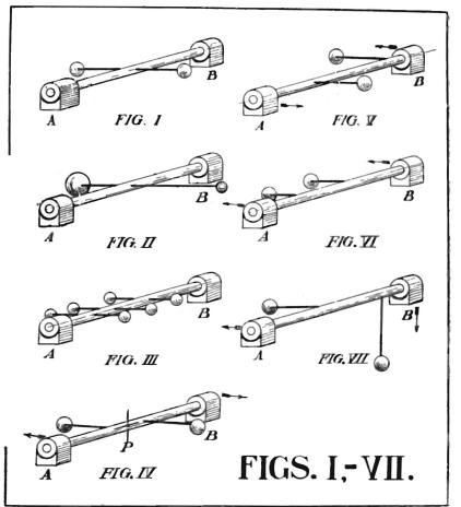
Suppose now we have two weights forming a unit placed as shewn in Fig. IV., and assume condition (a) is satisfied, i.e., it will be in static balance, clearly condition (b) is not, and if such a system is rotated, it will not be in dynamic balance, as the weights will set up centrifugal forces producing a couple tending to turn the shaft about some point P,
