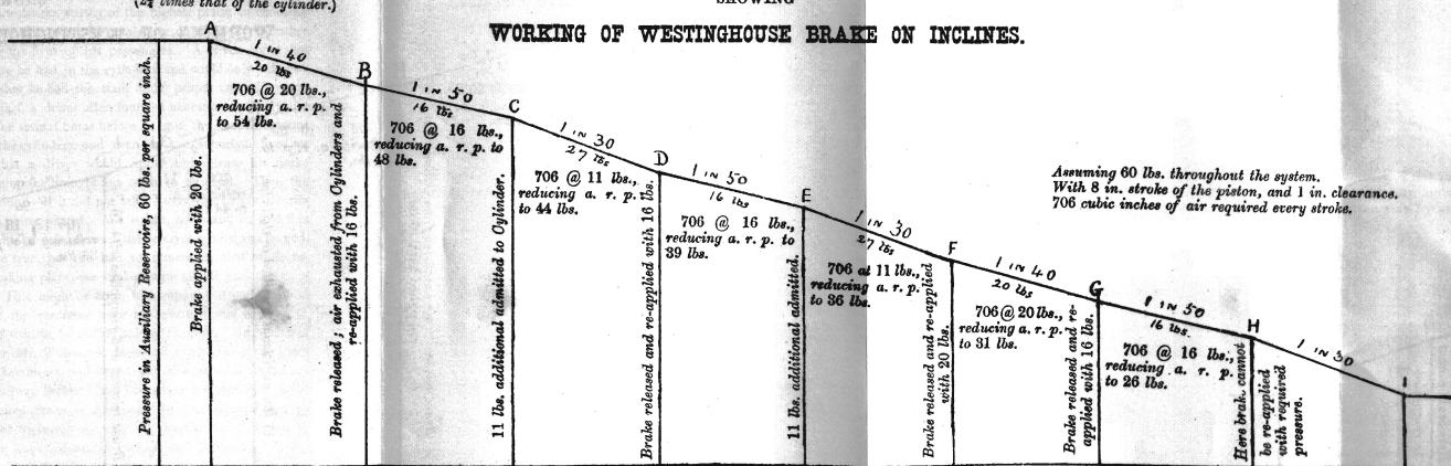
At H required controlling pressure should be 27 lbs., but only 23.6 lbs. can be obtained.
