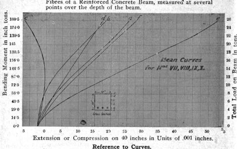
Fig 7.-Curves showing the Extension (or Compression) of Fibres of a Reinforced Concrete Beam, measured at several
