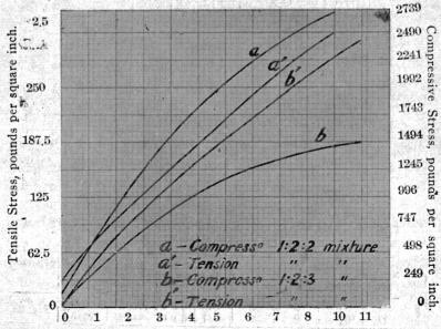
Compression per inch in units of .0001 inch. Extension per inch in units of .00001 inch.
