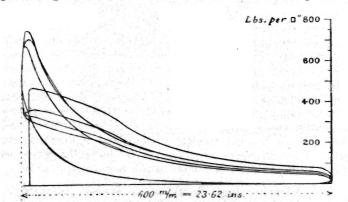
Fig. 8.—Full size Indicator Diagram from 160 B.H.P. Diesel Engine. Starting Card.
