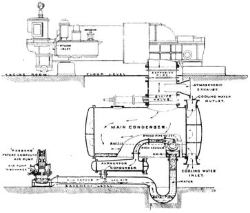
DIAGRAMMATIC ARRANGEMENT OF VACUUM AUGMENTOR. FIG. 7.
