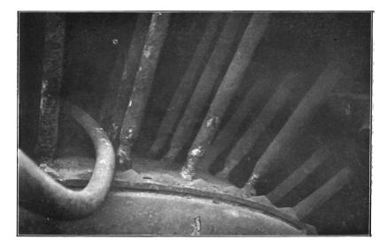
FIG. 13.—Furnace crown stays showing corrosion.
