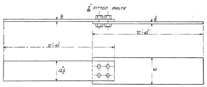
FIG. 16 C. FIG. 16.—Experimental Lap Joints. IV E.RS/ BIBLICIAN ) )
