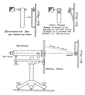
ARRANGEMENT OF TELESCOPE AND SCALE EMPLOYED TO RECORD MOVEMENTS OF THE MIRRORS ATTACHED TO THE TEST PIECE
