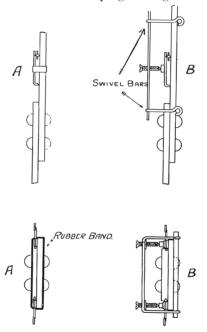
FIG. 18.—Methods of Pressing the Extensioneter Against the Test Piece.
