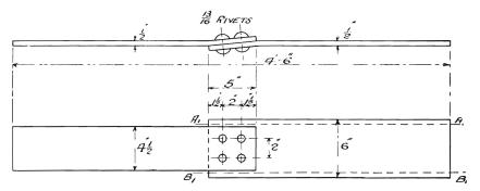
FIG. 16 B. LAP JOINT WITH JOGGLED PLATES
