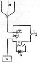
Circuit with electrolytic detector. Fig. 15.
