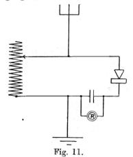
The next step, as shown in Fig. 11, was to put it in a derived circuit, shunting it round a variable tuning inductance which was used to bring the air wire to its proper period for reception.
