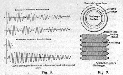
The office of this form of gap was to lock off the condenser circuit the instant the first transfer of energy had taken place to the air wire circuit, and thus prevent the second pendulum from returning any of its energy to the first.
