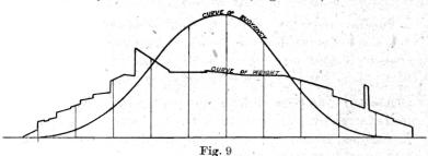
of the ship must be fair, and therefore regulating the buoyancy to suit the weights is out of the question; the alternative is to regulate the strength of the structure at and about such variations, which is now commonly done, as distinguished from the old method of uniformly graduating the scantlings from half or three-fifths length towards the ends.
