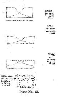
PLATE No. 12: Showed a set of cards taken off the engines whilst under duty. The H.P. cylinder showed 90.56 I.H.P., the Intermediate Pressure 87.29, and the low pressure cylinder 99.47, which gave a mechanical efficiency of 93.2 per cent.
