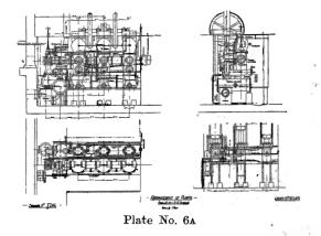
PLATE 6A: A feed water heater was placed on the exhaust steam pipe between the low pressure cylinder and the condenser. having a number of solid drawn "U" tubes, expanded into a cast iron header. This heater had a capacity equal to heating all the feed water to within two degrees of the temperature of the exhaust steam, and was provided with the usual bye-pass valves for throwing it in and out of action.
