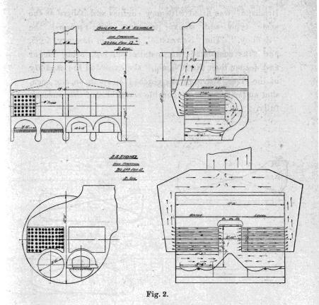
Figs. I. and II.—These vessels were all of iron, propelled by paddle wheels, fitted with wooden floats, and of the feathering type. The engines were low-pressure oscillating, carrying a steam pressure of 30 lbs. per square inch.
