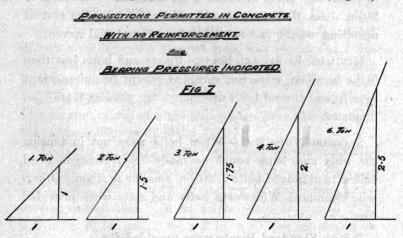
The resultant of all forces was to fall within the centre third of the foundation, and the average pressure was not to exceed half the maximum bearing pressure allowed. The following formula assisted in estimation :---
