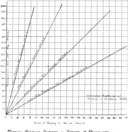
MICHELL BEARING DIAGRAM OF SPEEDS & PRESSURES WITH OIL OF VARYING THICKNESS Fig. 3.
