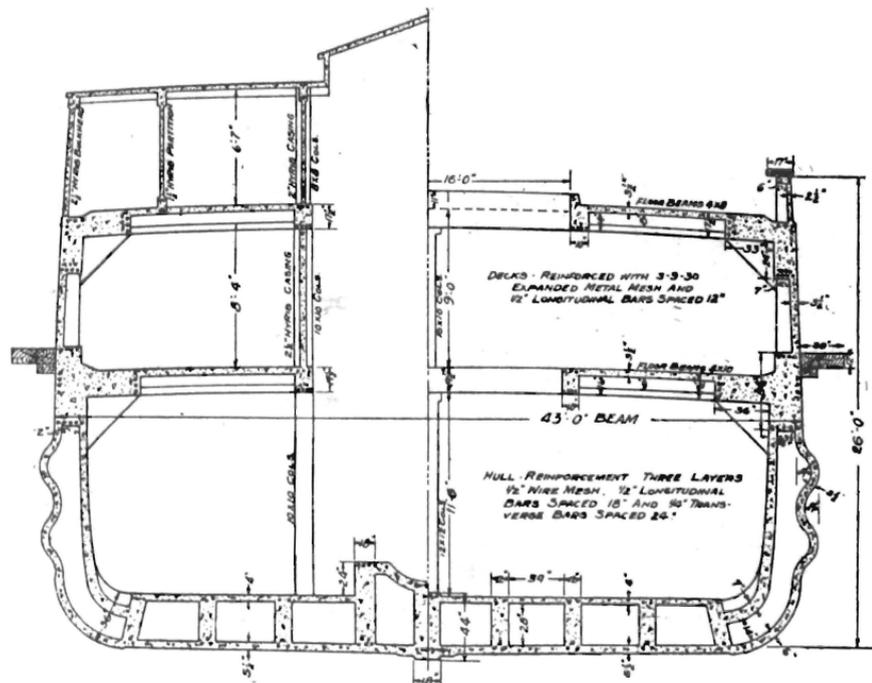
Fig. 5.—Reinforced Concrete Freighter. "Marine Engineering," page 302.
