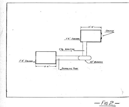
In these experiments the greatest difficulty I met was to devise a means of making the wooden boxes airtight, and keeping them in such condition. I finally decided to provide all joints with a tongue, and, after screwing up tight, run in a quantity of marine glue. This gave satisfactory
